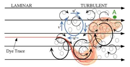
A schematic diagram showing the movement of a fluid from the left to the right. It starts with laminar flow (on the left) and then it quickly becomes turbulent flow (on the right), which contains a lot of eddies (swirling structure). The injected red dye on the left shows the fluid motion. The flow enters the turbulent area and it is carried by the eddies to reach point A.
